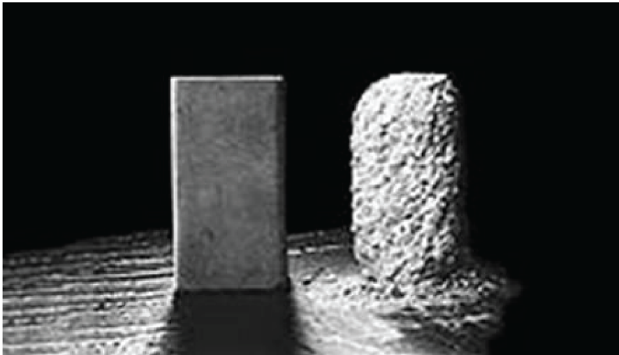
Figure 7. The result of the impact of 10% hydrochloric acid on concrete (sulfur - left, cement - right)
